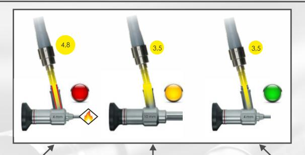
You use a thick light-guide with diameter of 4,9 mm. You use the thin optics with diameter of 3,5 mm of light entry.
